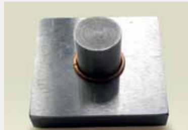
Test piece before brazing
