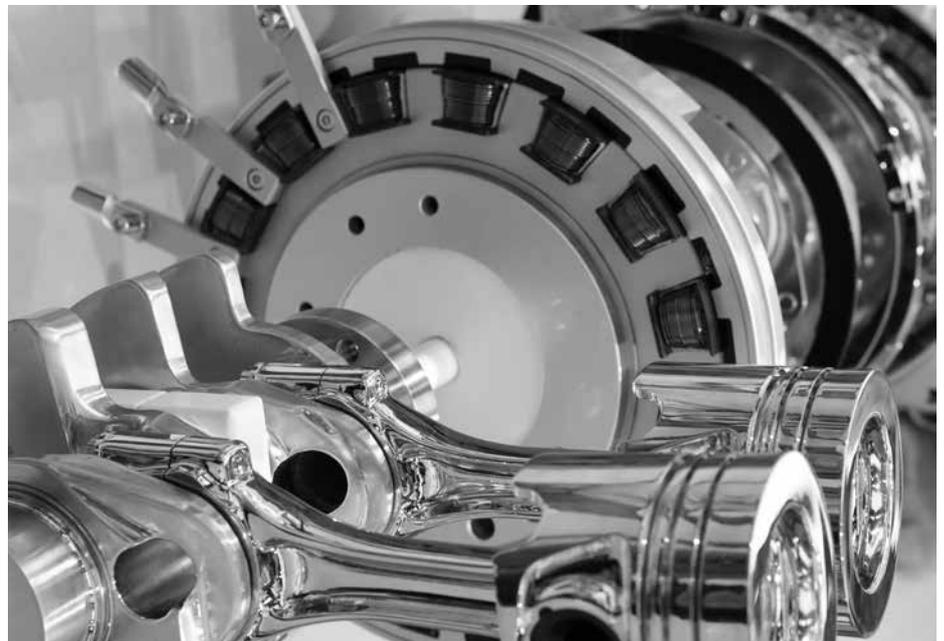
High-efficiency hybrid vehicle engine with electric motor.
