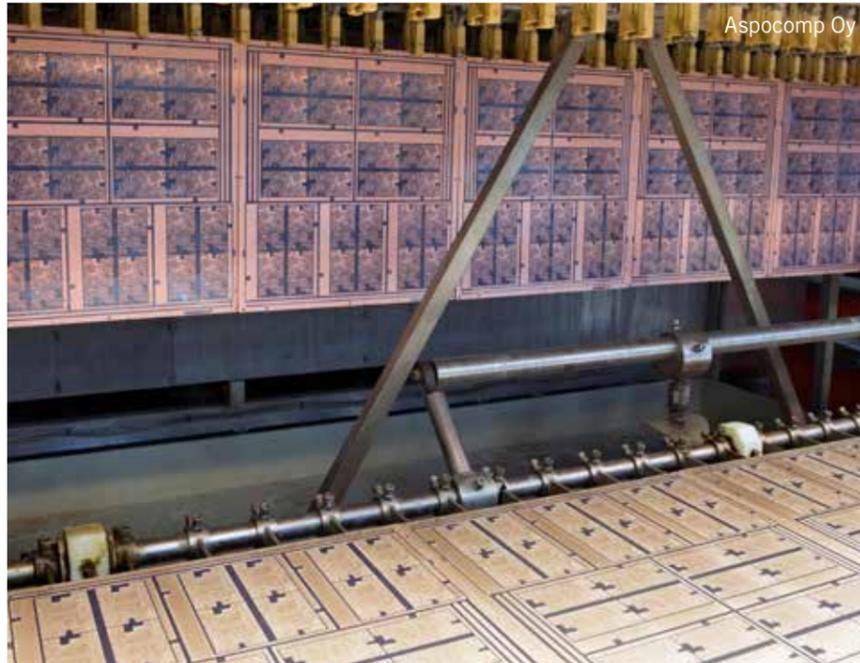
Printed circuit board plating
