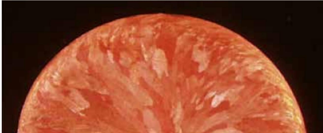
Figure 1. Luvata's anode balls contain large cast grains.
