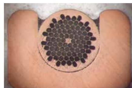
MRI wire-in-channel (WIC) conductor with 84 filaments
