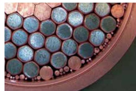
Multifilament billet assembly
